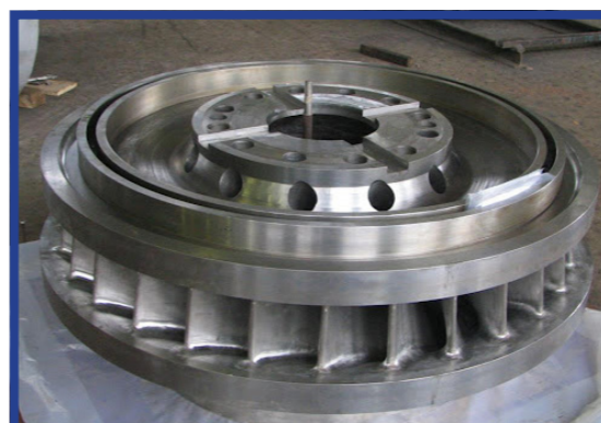
TUA BIN FRANCIS TURBINE GENERATOR
